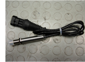
Pavement temp. Sensor
